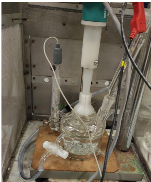
Figure 2.7 Single cell setup housing RRDE GC/Pt tip (center), SCE electrode in a Luggin capillary (left) and a Pt counter electrode in a bridge equipped with a Vycor frit.
