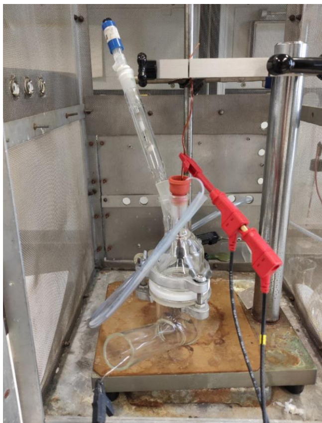
Figure 2.8 Two compartments cell with working and reference electrode on the top and counter electrode at the bottom compartment. The two were separated by a Nafion 117 membrane.
